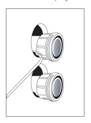
There should still be approx. 15mm from the inside of the coupling to wall to allow the cover plate to be installed.
