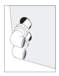
Measure the distance from the wall to the centre of the elbow. This is the centrepoint for the pump to be installed on.
