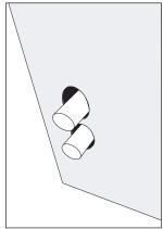
With the bath in position, and the pipes through the wall, cut the pipes to be protruding the wall by 50mm, and glue on the male manifold couplings.
