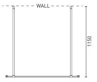
NOTE 1150mm wall brace can be cut down to size
