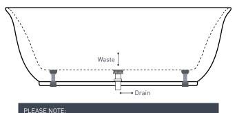
Connect the waste directly to the drain. A flexible bath connector cannot be used with the Lola 1700 due to the waste clearance being under the 85mm required for a connector to be used.
