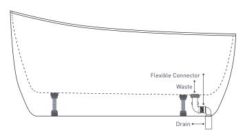
OWA004 Decina Flexible Connector + Pop-Up Waste Min. clearance 100mm OWA005 Decina Flexible Connector Min. clearance 80mm
