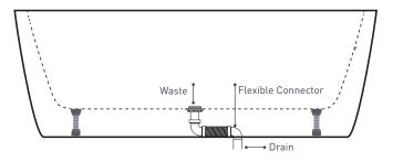
OWA004 Decina Flexible Connector + Pop-Up Waste Min. clearance 100mm OWA005 Decina Flexible Connector Min. clearance 80mm
